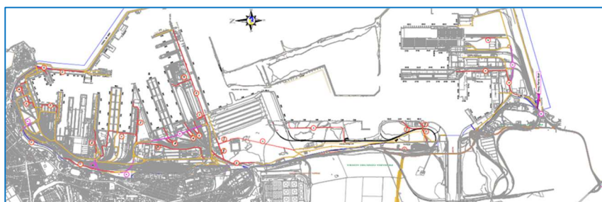
Figure 11.4: Implementation of the Master Plan for road and access infrastructure in the port of Constantza (rehabilitation, modernization, extension), including road bridge to the artificial island
