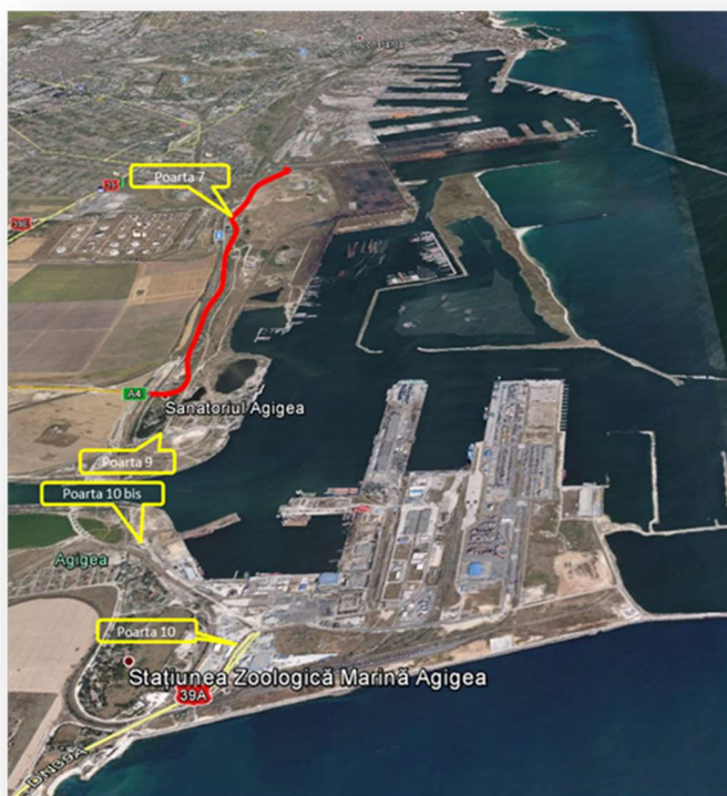
Figure 11.1: The extension to four lanes of the road between Gate 7 and the intersection of the objective “Road bridge at km 0 + 540 of the Danube Canal - Black Sea” with the road that connects Gate 9 and Gate 8 to the northern part of Constantza Port
